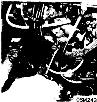
ADJUSTING DECELERATION SPEED SCREW
