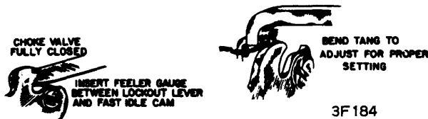
SECONDARY LOCKOUT ADJUSTMENT
