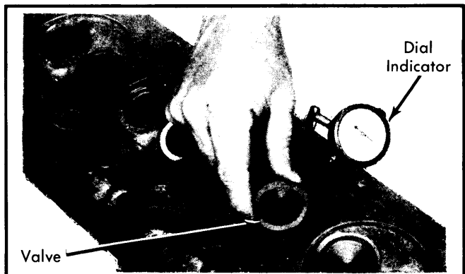
Fig. 2 Measuring Valve Stem-to-Guide Clearance.
