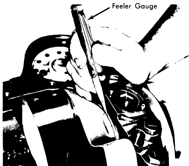
Fig. 8 Using Feeler Gauge to Check Crankshaft End Play
