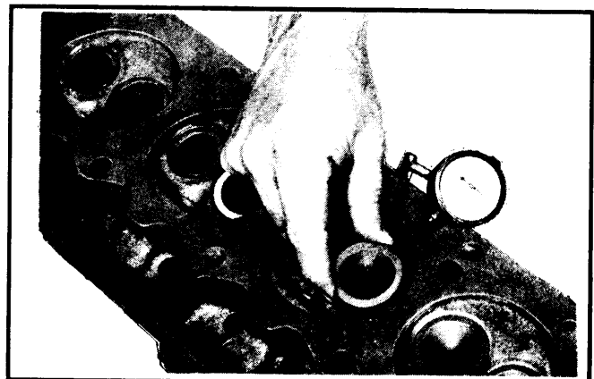
Fig. 2 Measuring Valve Stem-to-Guide Clearance.
