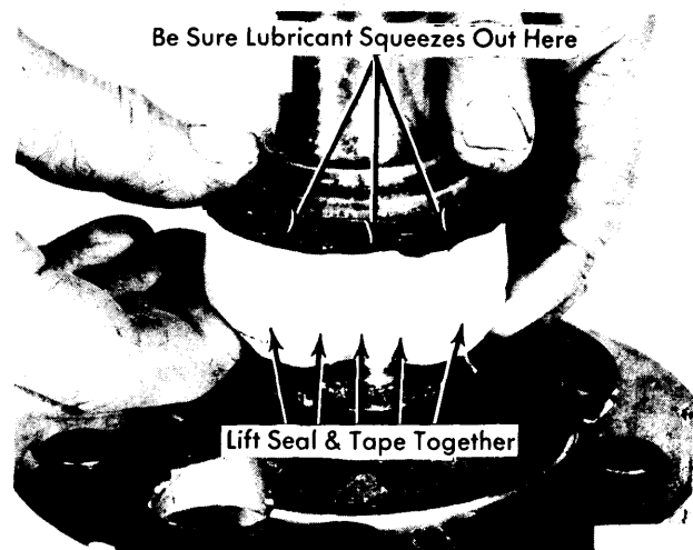
Fig. 2 Correct Procedure for Lubricating Installed Bearing 2) On disassembled axle, install retainer and carefully position seal on machined seat on axle. Press bearing onto shaft making sure that cup rib ring is towards flange end of shaft (see illustration). Press new bearing retainer ring on axle shaft with narrow end toward splined end of shaft. (Bearing and retainer can be pressed on at same time). Bearing and retainer must be pressed into seat on shaft so that a .0015" feeler gauge cannot be inserted between seat and bearing or between bearing and retainer.
