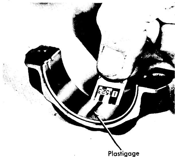
Fig. 10 Using Plastigage Method to Check Bearing Clearance
