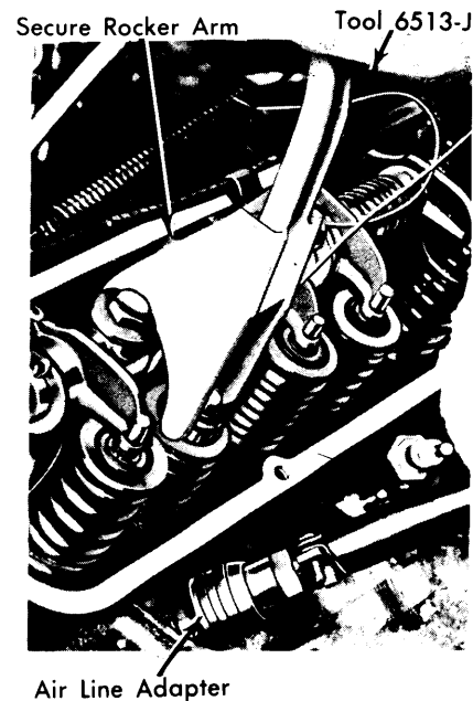
Fig. 6 Compressing Valve Spring for Removal
