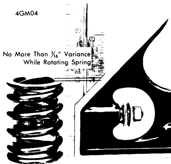
CHECKING VALVE SPRING SQUARENESS
