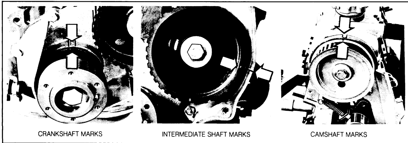
Fig. 2: Timing Marks for Crankshaft, Intermediate Shaft and Camshaft
