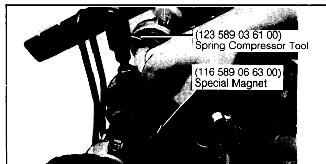
Fig. 4: Removing Valve Keepers
