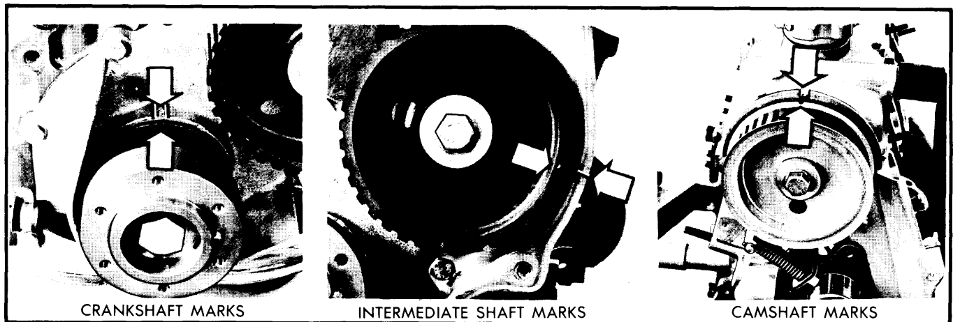
Fig. 2 Timing Marks for Crankshaft, Intermediate Shaft and Camshaft
