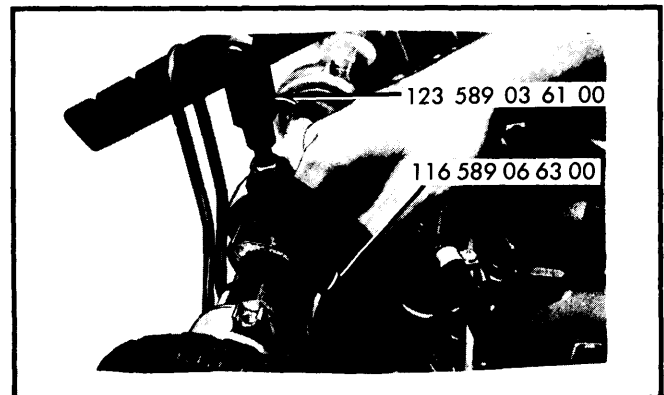
Fig. 4 Removing Conical Valve Key Halves (Keepers)
