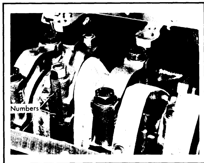
Fig. 9 View Showing Connecting Rod Cap Installation
