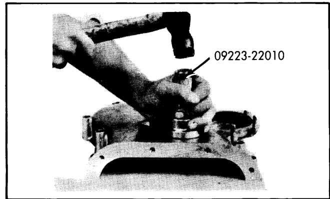
Fig. 12 Using Special Tool to Install Oil Seal in Front Cover
