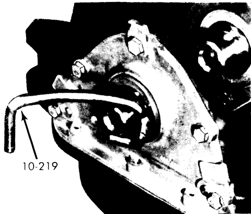
Fig. 6 Using Special Tool to Remove Front Oil Seal
