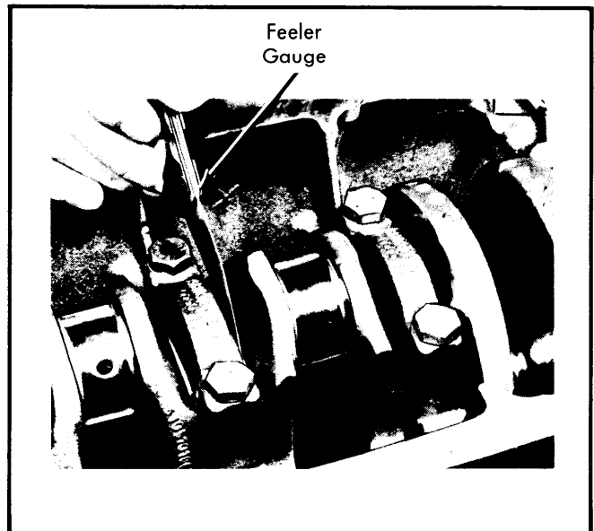
Fig. 10 Measuring Crankshaft End Play
