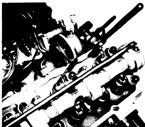
Fig. 4 Dial Indicator Installed
