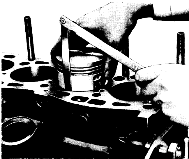
Fig. 8 Using a Feeler Gauge to Check Piston-to-Cylinder Wall Clearance
