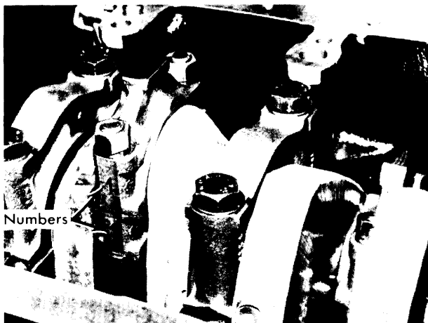
Fig. 4 View Showing Connecting Rod Cap Installation
