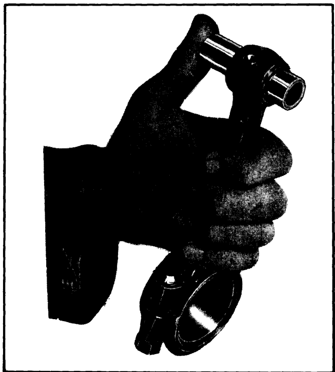
Fig. 6 Thumb Pressure Piston Pin Fit
