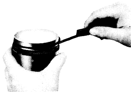
Fig. 10 Using a Feeler Gauge to Measure Ring Clearance
