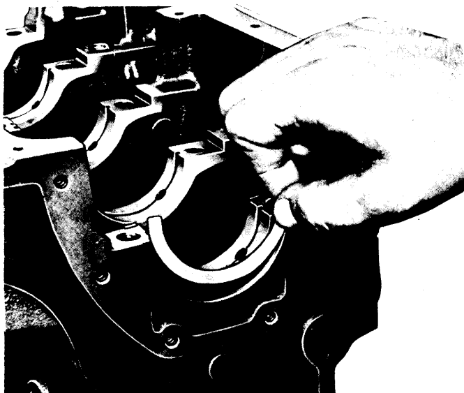
Fig. 9 Fitting Crankshaft Thrust Washer to Block
