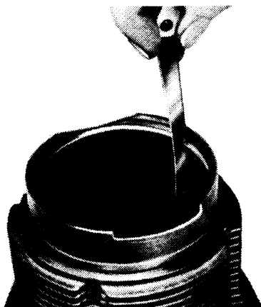
Fig. 7 Using a Feeler Gauge to Measure Piston Ring Gap
