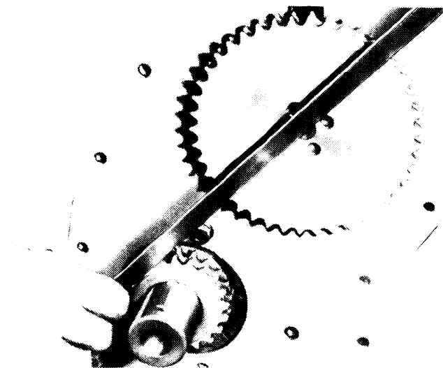
Fig. 7 Using a Straightedge to Check Sprocket Height
