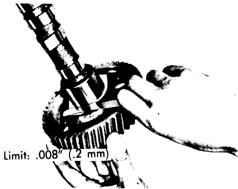
Fig. 16 View Showing Typical Camshaft Bearing Removal (No. 3 & Rear Shown)
