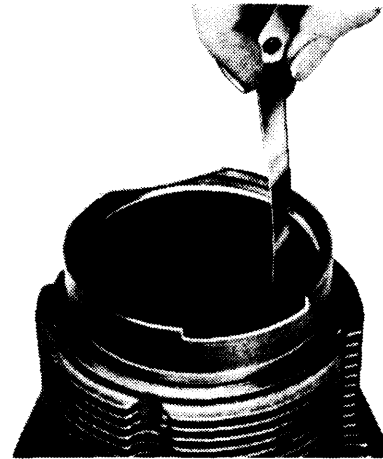
Fig. 4 Measuring Ring Gap with Ring in Cylinder
