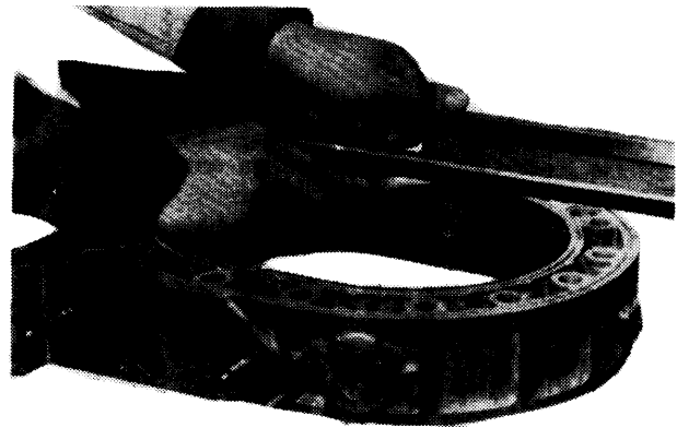
Fig. 10 Measuring Rotor Housing for Distortion
