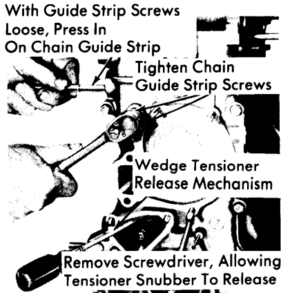
Fig. 7 Adjusting Timing Chain Tension
