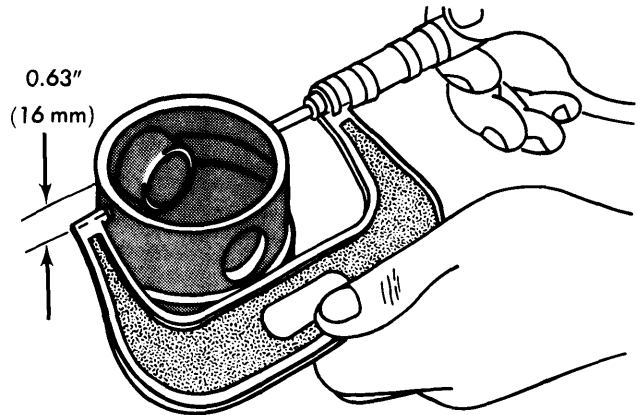
Fig. 4 Correct Procedure to Measure Piston Diameter
