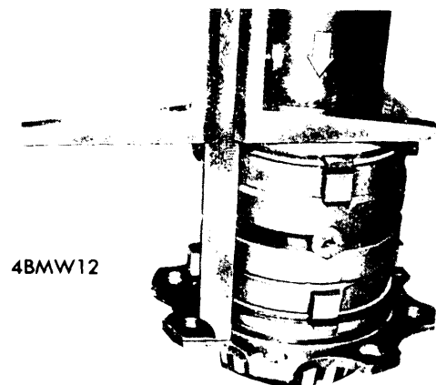
MEASURING CLUTCH ASSEMBLY INSTALLED HEIGHT (WITH PRESSURE APPLIED)
