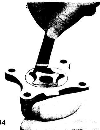
CHECKING ROTOR LOBE CLEARANCE
