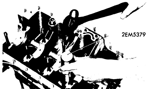
CYLINDER LINER REMOVAL
