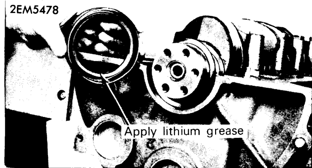
REAR MAIN BEARING OIL SEAL INSTALLATION
