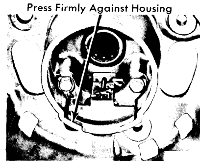
Fig. 9 View Showing Brush Lead Wire Routing
