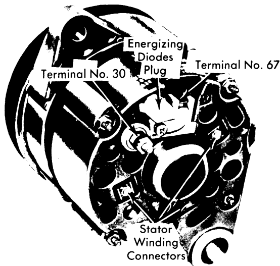
Fig. 2 Marelly Alternator Test Points
