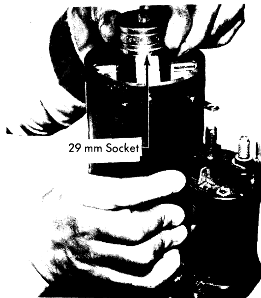
Fig. 2 Holding Brushes in Position While Removing Field Frame
