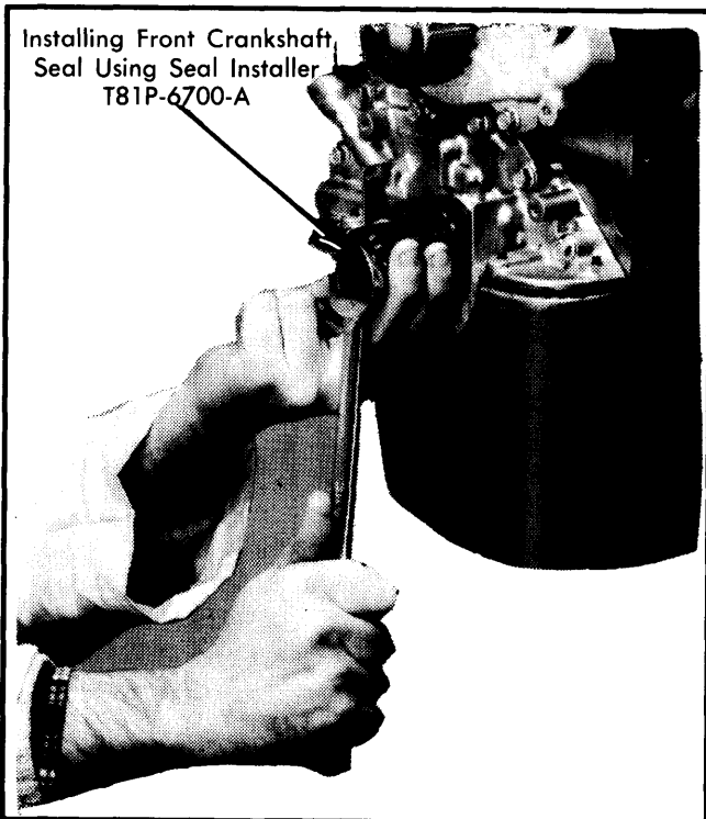
Fig. 8 Installing Front Crankshaft Oil Seal
