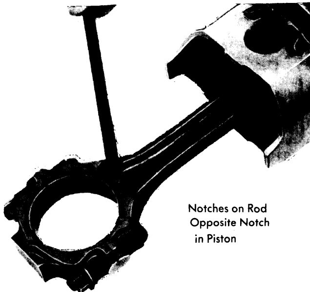
Fig. 6 Making Sure Connecting Rod and Piston Assembly Are Properly Indexed
