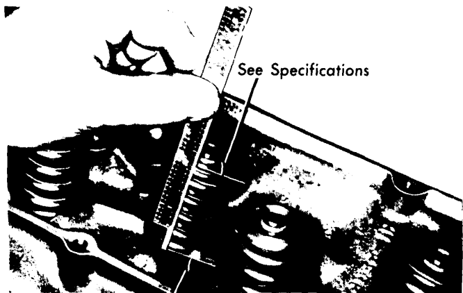
Fig. 3 Valve Spring Installed Height
