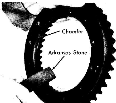
Fig. 5 Cutting a Chamfer on Ring Gear Using a Cutting Stone
