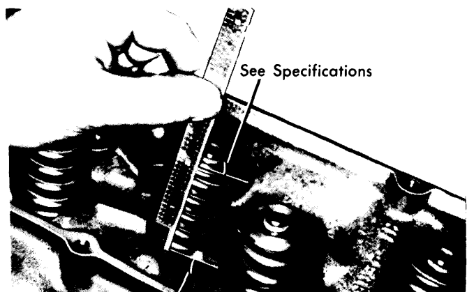
Fig. 3 Valve Spring Installed Height
