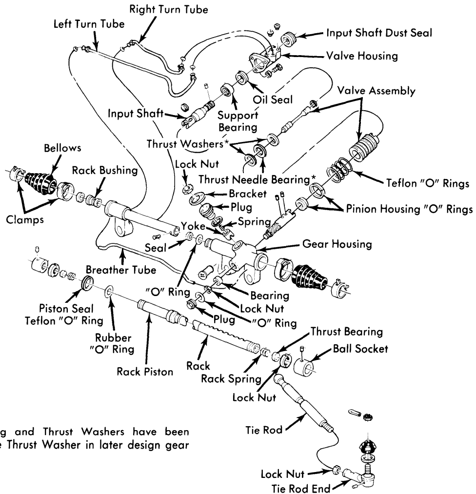
Fig. 9 Power Rack & Pinion Steering Gear
