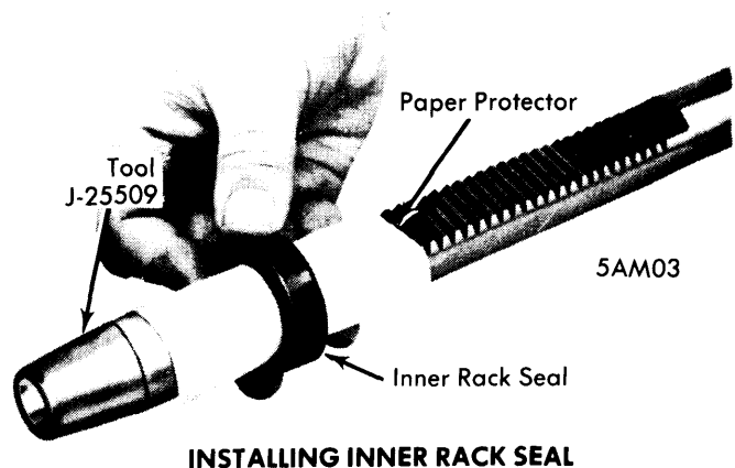
INSTALLING INNER RACK SEAL
