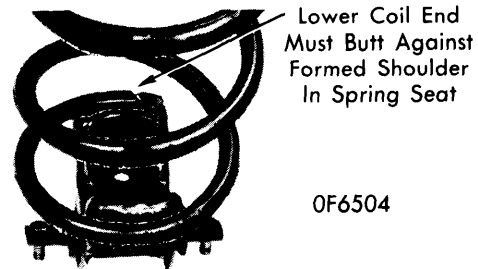
LOWER SPRING SEAT INSTALLATION
