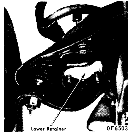
INSTALLING LOWER RETAINER OF SPRING COMPRESSOR TOOL
