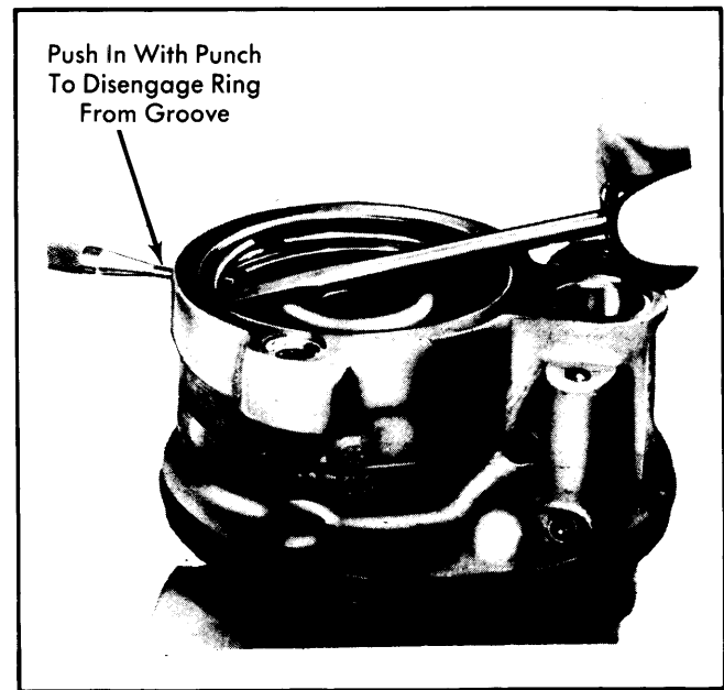
Fig. 2 Disengaging and Removing Retaining Ring for End Plate of Pump
