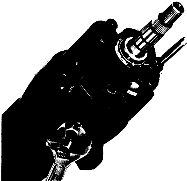
Fig. 14 Removing Pivot Pins from Column
