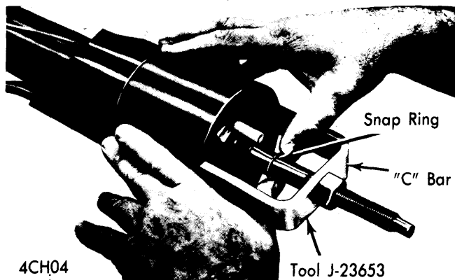
INSTALLING LOCK PLATE SNAP RING
