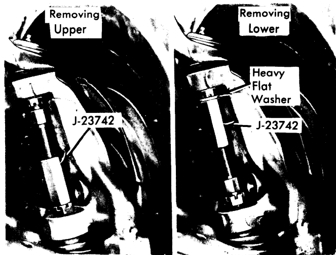
REMOVING BALL JOINTS 4CH03
